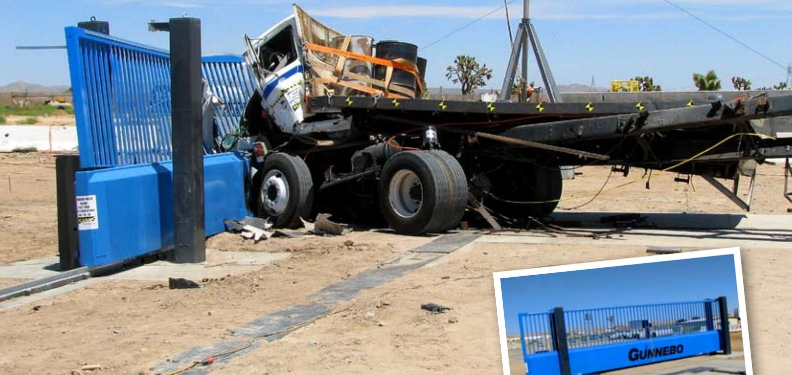
*Tracked Gate M50 successfully passed the ASTM M50 test – almost unique for a gate of its size.*
