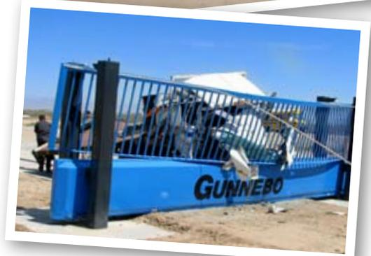
*To pass the M50 test, the gate had to stop dead a truck weighing over 6700kg travelling at 50mph (80km/h) and prevent it from penetrating further than one metre.*
