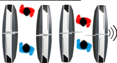
Wrong way direction/intrusion attempt
